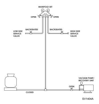
Figure 7-7. Recovery/Evacuation Connections
